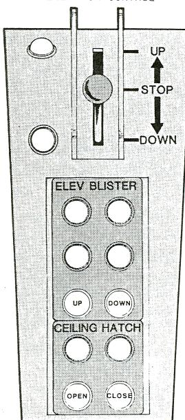
The Jupiters elevator is designed not only to transport personnel and equipment between decks, but also as an elevating platform for the navigation site. The site, mounted in a blister or bubble dome, will be raised through a ceiling hatch for a clear view of the stars.
