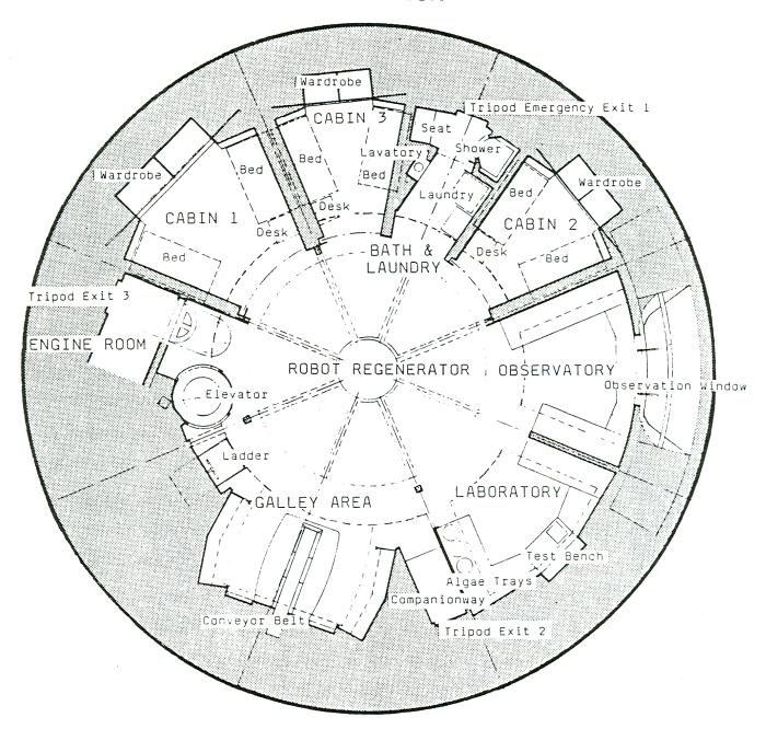
This is the primary living deck for the space family, it contains sleeping quarters, galley, laboratory and the spaceships "extra" crew member—an environmental control Robot. Landing gear will extend from the lower deck to provide access to the surface of the new planet. An Observatory will provide a clear view of the future camp site and farm.
